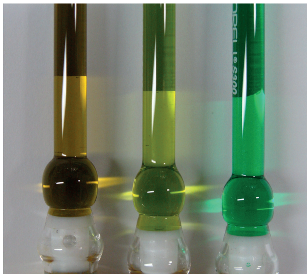
Figure 5. Characteristic colors of dichloromethane solutions of the new copper carbene complex 2 Cu (left), of the new silver carbene complex 2 Ag (middle) and of the already published gold carbene complex 2 Au (right). [14]
